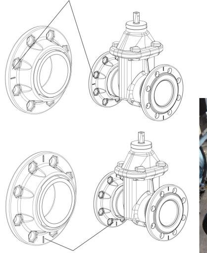
horizontal marking: Loose flange can be slid over the lock
