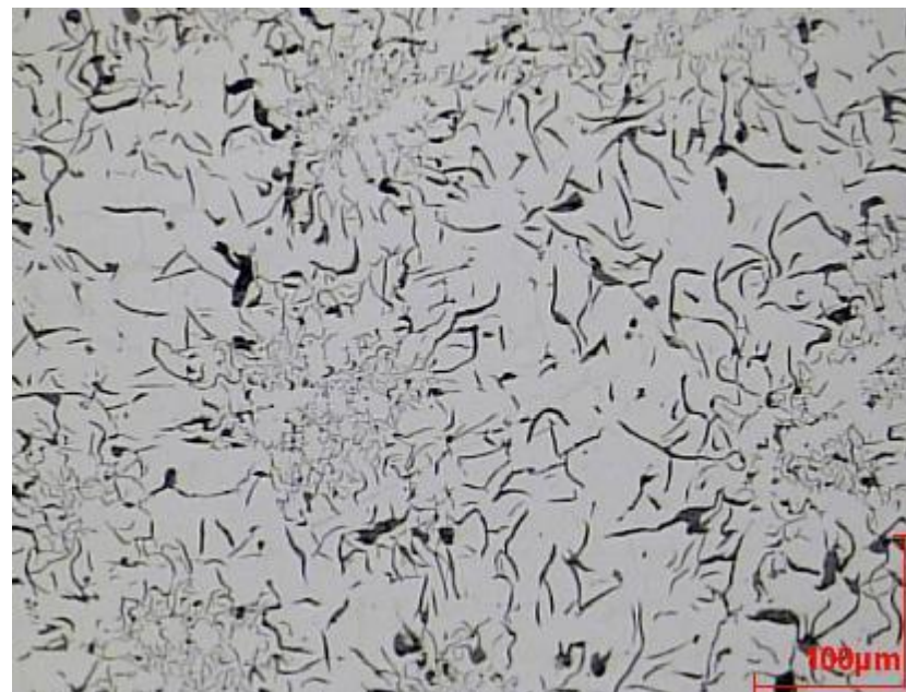
The structure of Düker cast iron with flake graphite under the microscope
