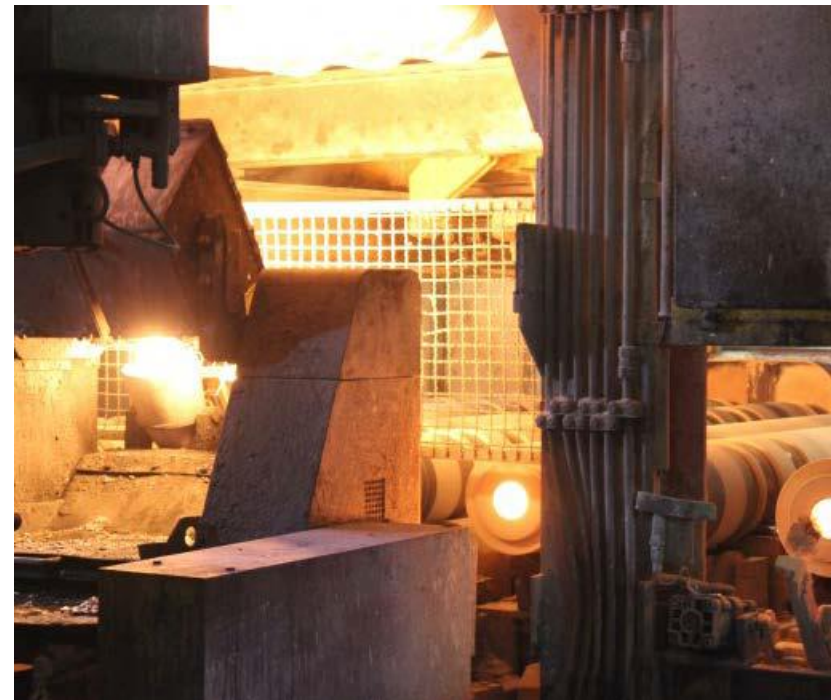
Centrifugal casting plant: pouring into the rotating pipe molds
