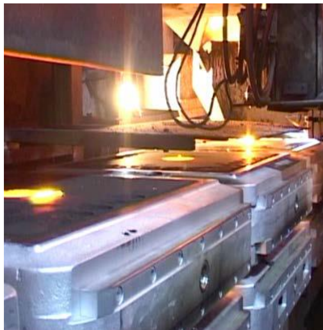
Moulding plant: pouring into the sand molds
