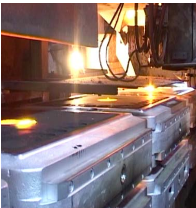
Moulding plant: pouring into the sand moulds
