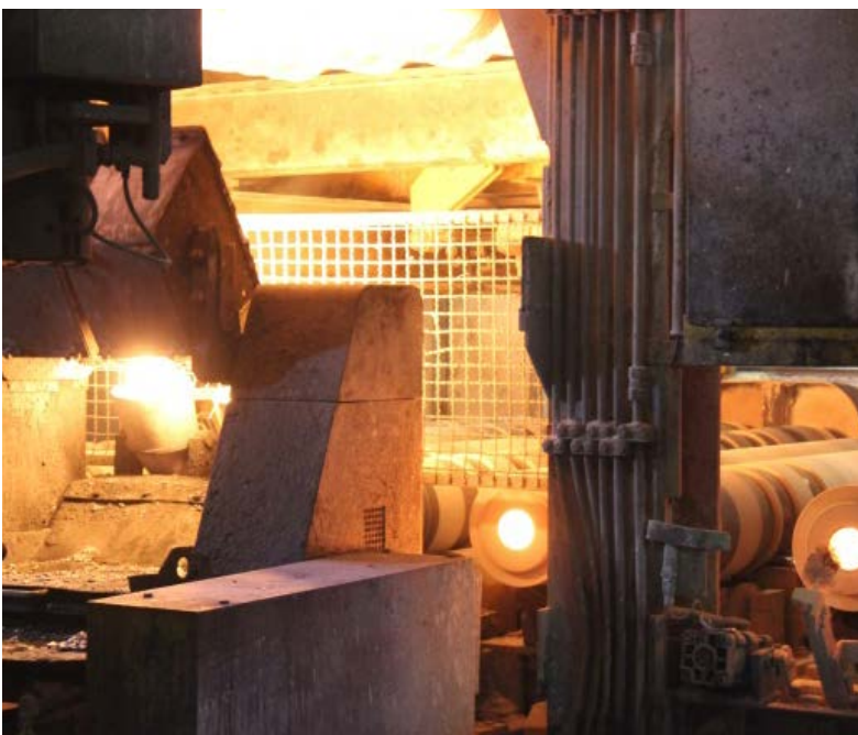
Centrifugal casting plant: pouring into the rotating pipe moulds
