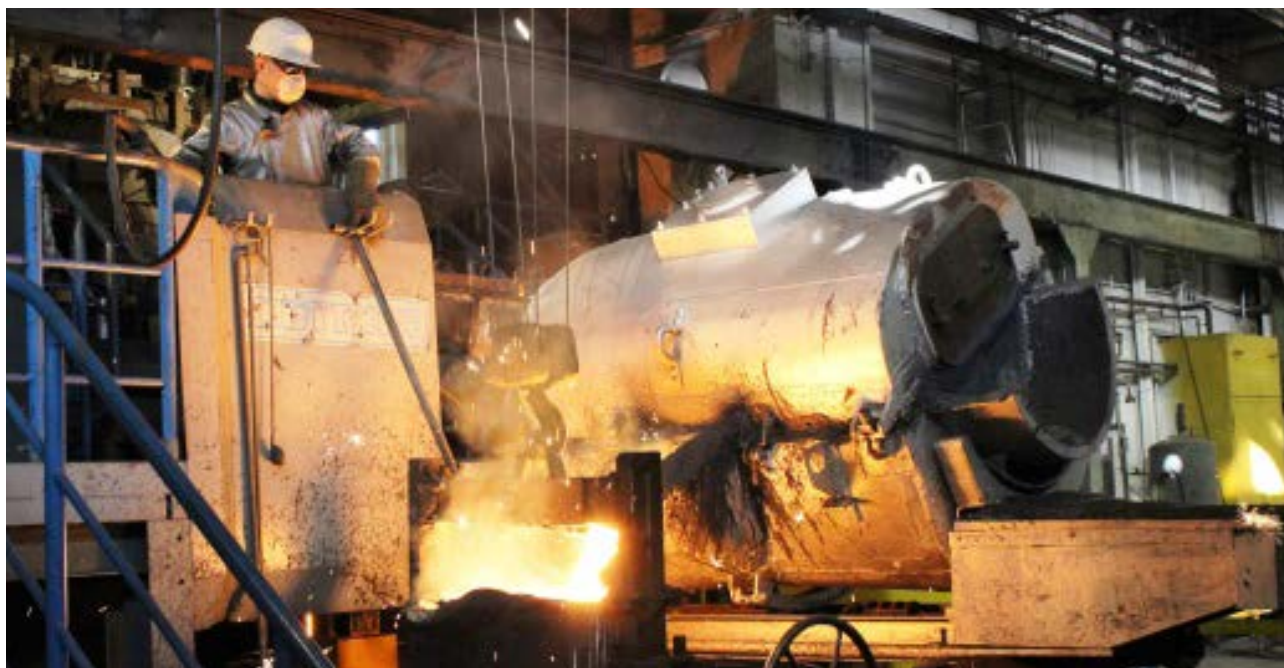
Melting shop: Withdrawal of liquid iron from the collector
