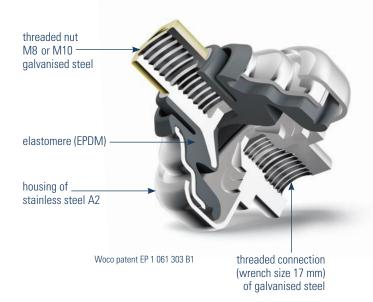
The acoustic decoupler can face the bracket with any of its two sides.
