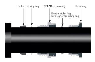
Enables mounting without block strapping and the thrust-resisted connection with flanged sockets and collars. Screw ring and SPEZIAL-Screw ring are delivered in blue-grey colour.
