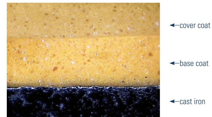
polished cutting of the protec inside coating
